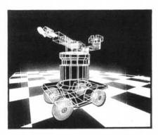
Computer FX is a newly established London computer graphics facility specialising in the production of 3-D animation sequence. The system was developed in-house and is completely interactive. It is based on IMI vector-refresh hardware which allows complex animation in real-time. Over 100 objects, each having 9 degrees of freedom can be animated simultaneously.
